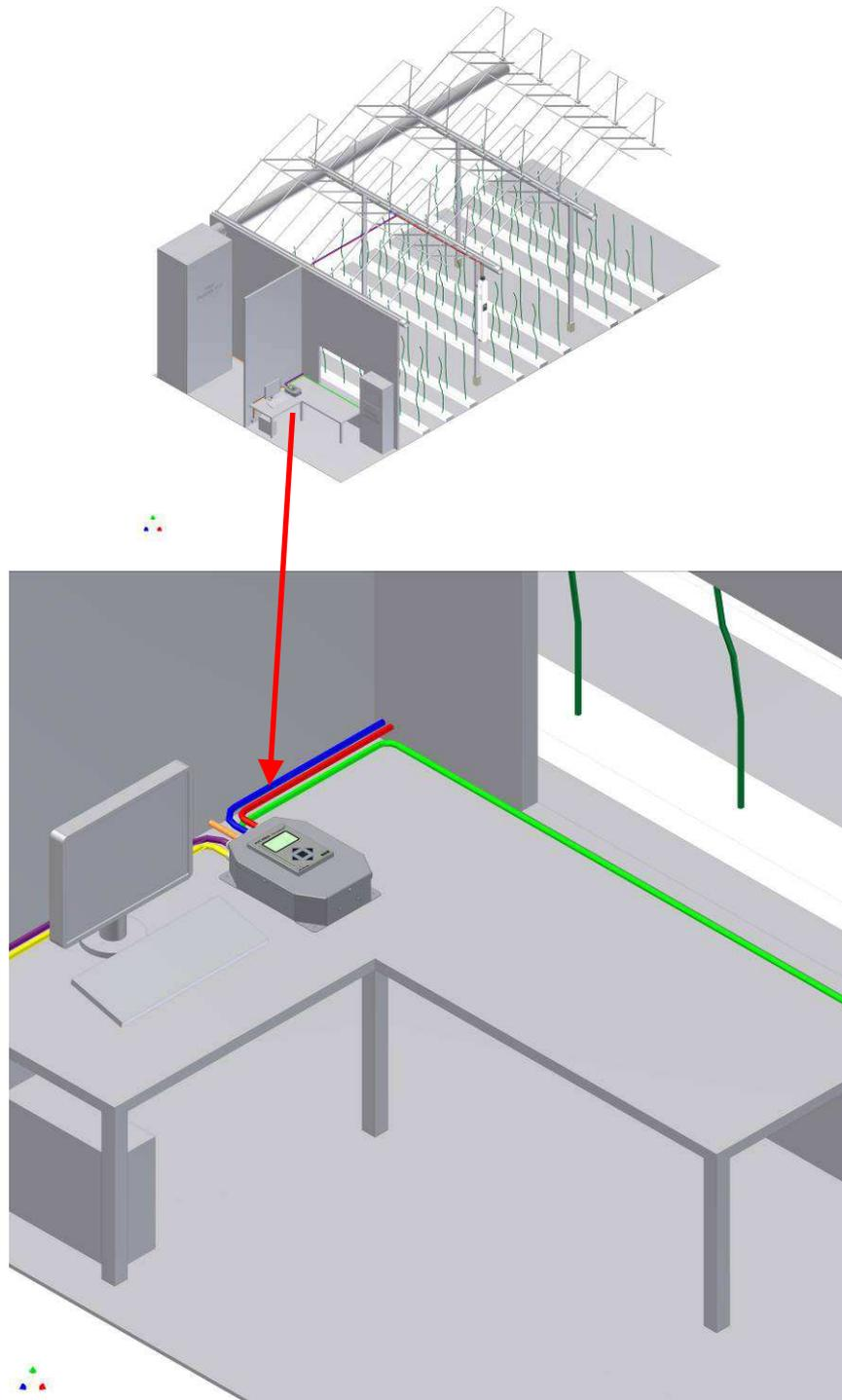
Figure 4: Demonstration example inside the office with the IO-BOX connected to the climate computer.
