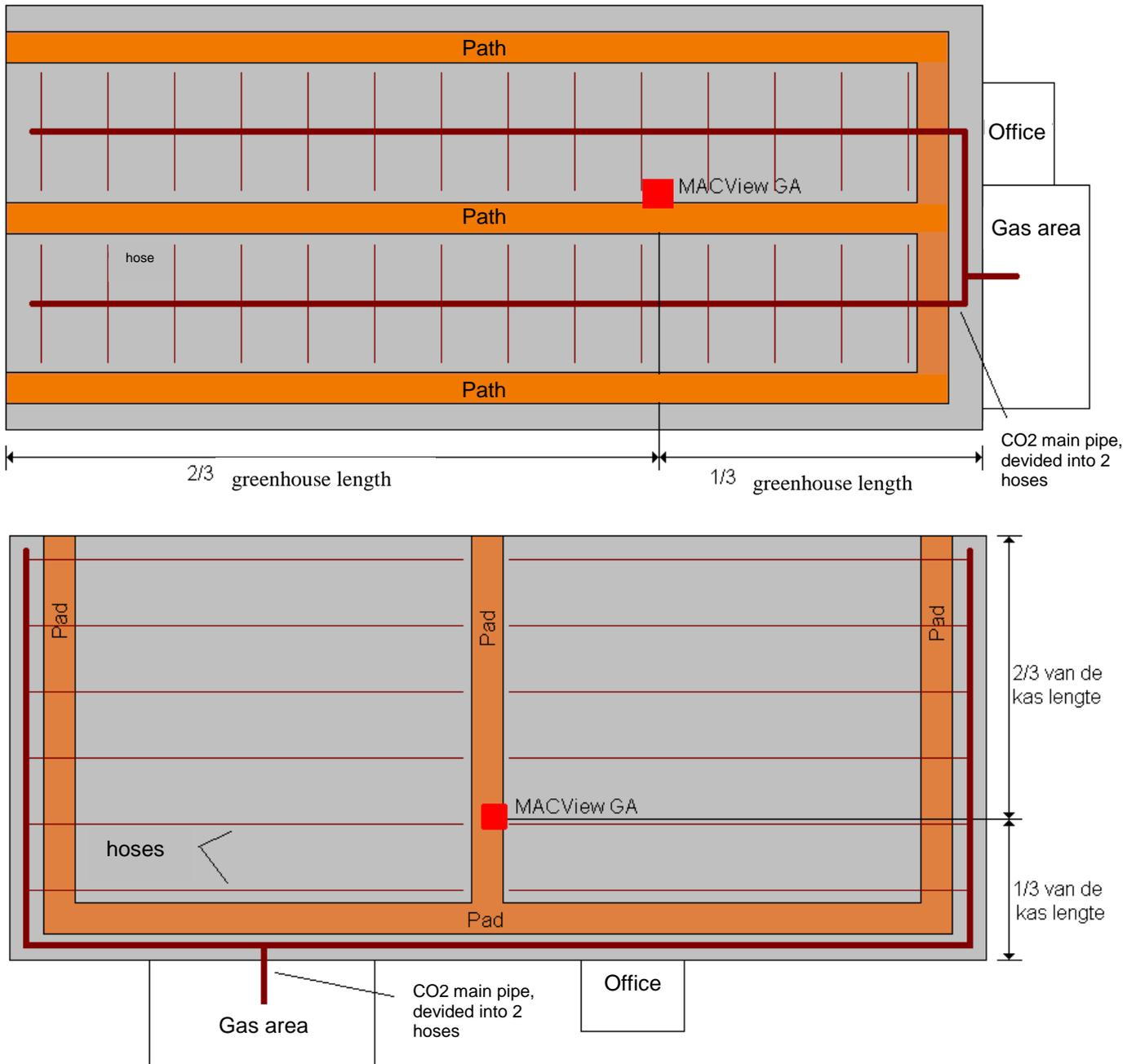
Figure 5: Two examples of CO2 dose units. The position of the MACView® GA is given by the red sign.
