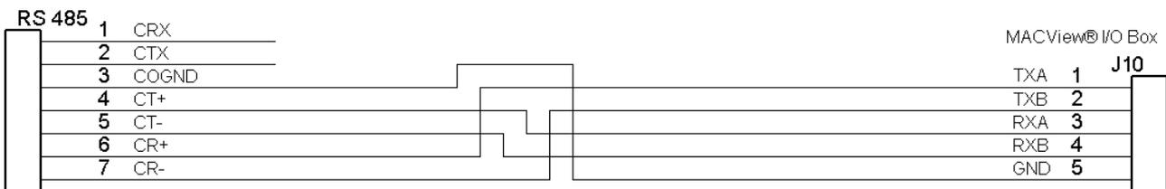
Figure 6: Wirings of RS 485
