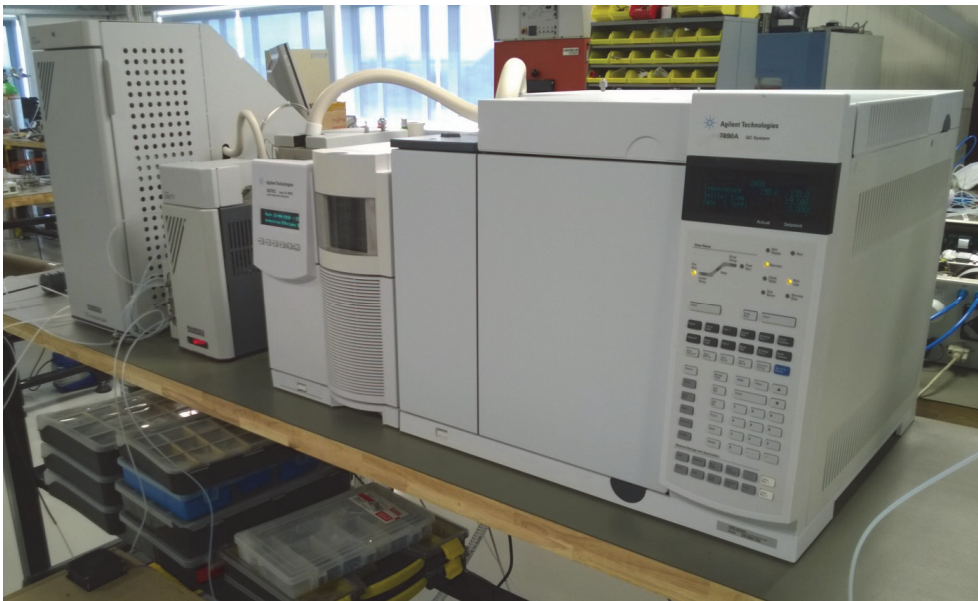
Figure 2: Thermal Desorption Gas Chromatograph Mass Spectrometer (TD-GC-MS) at the test set up.
