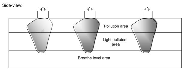
Although we dissuade placing a sensor in the extraction cone of the fan, it can be considered in situations when it is impossible to choose another place, because there are to many harassing effects. In that case we advice to place the sensor close to the fan or ventilator.
