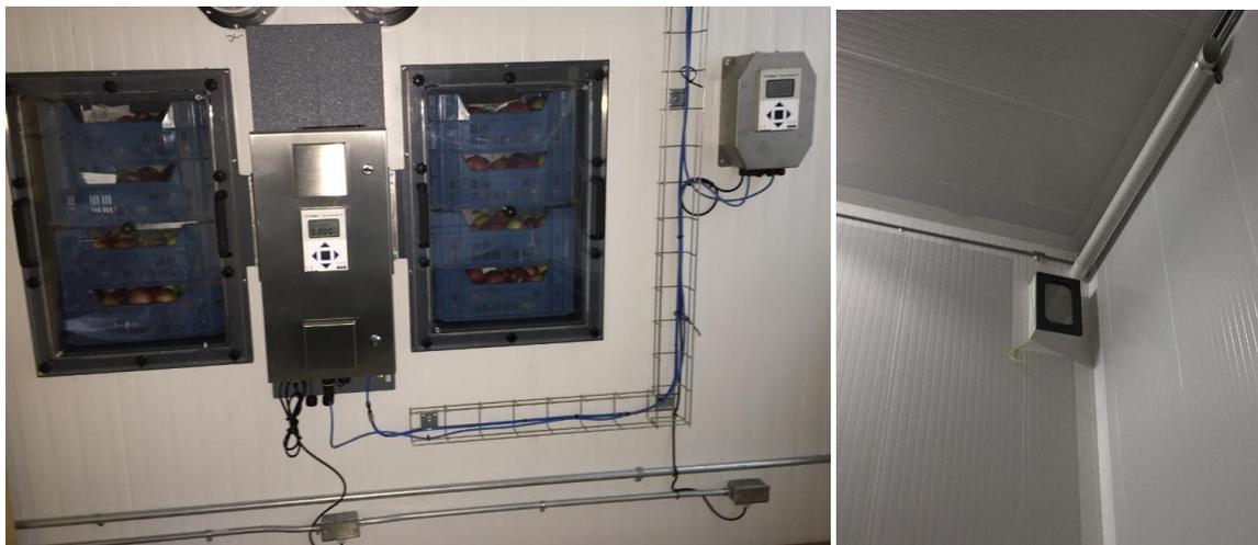
The top of the measuring box is made out of a pvc plate. This pvc plate is working as a flange for the measuring box. Around the opening in the top of the flange a channel is milled in which a large rubber ring is placed for gas tight closing of the transparent lid. The lid can be easily fixed and removed by 10 screws.
