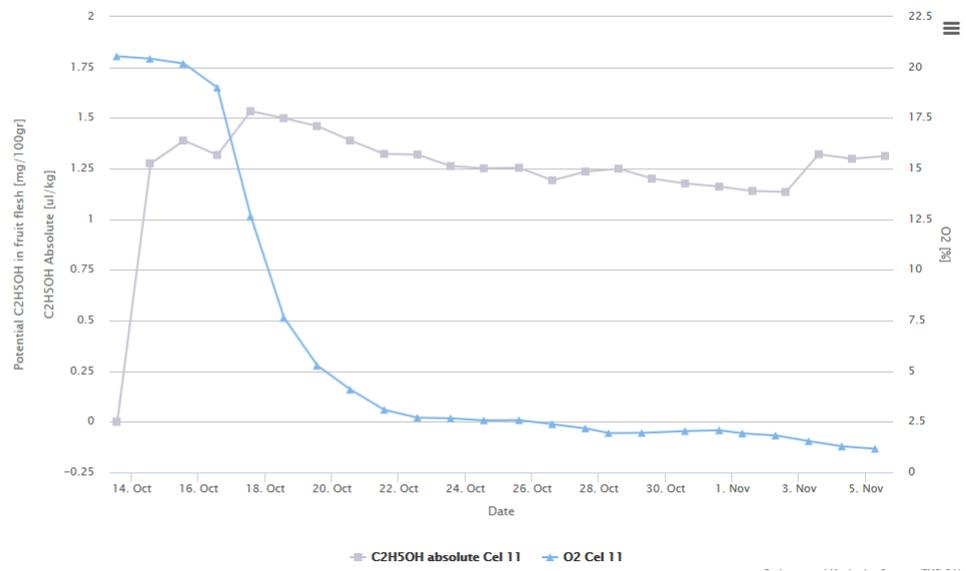
For the value 'Potential mg ethanol / 100gr fruitflesh' we have developed an algorithm in which the measured ethanol value in the air is recalculated based on the present weight of the sample into value of 'Potential mg ethanol / 100gr fruitflesh'.
