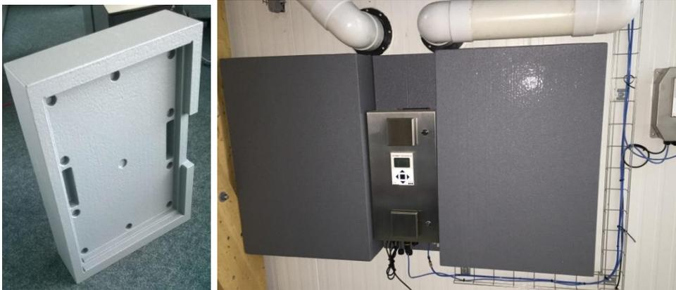
The measuring boxes can contain each a maximum of 4 plastic boxes. In the frame of the measuring box 2 x 2 boxes can be placed.
