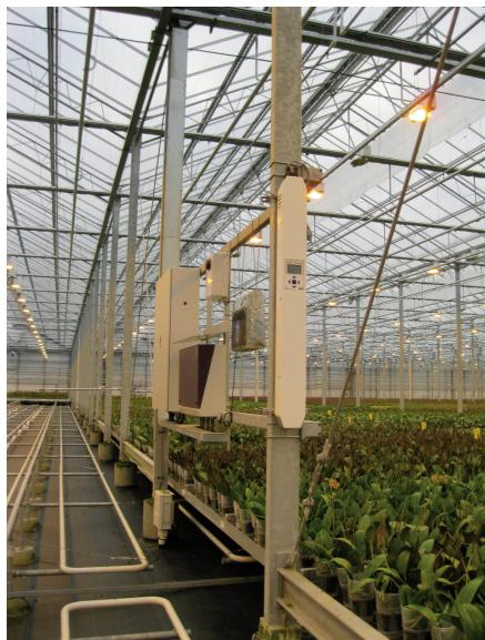
The MACView®-Greenhouse Gas Analyser assists the grower by interpreting the way the gas conditions in the greenhouse are in relation to the valuable product in the greenhouse.
