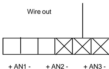
The plug must be placed on the 3 positions marked with a cross. The drawing represents the view from the inside of the lid. The lid is placed upside down with the display down and the electronics above.
