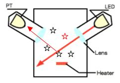
Figure 1 - Model of dust sensor
